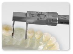
$\mathbf{OUT}$  shows the determined outside dimension (Ø 1.5 mm),  $\mathbf{IN}$  shows the inner diameter.
