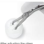
After adjusting the pliers, tips should be moistened with diamond powder
