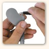
Pull in the tip with the **ZEPF** Safety Key. With the other end, proceed as before. To set the tips, it is better to use two Safety Keys.
