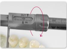
Locating screw for a safe fixation of the measured result.
